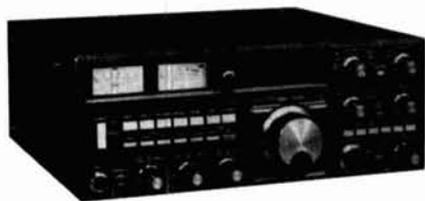
hf transceivers, the FT-726R includes an SSB speech processor, i-f shift, variable i-f bandwidth tuning, i-f noise blanker, RIT, multimode squelch, and a receiver audio tone control. A CW filter, DTMF encoding microphone (YM-
