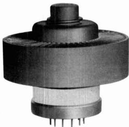
Height of the 3CX800A7 above the socket plane is only 2-1/4 inches (5.7 cm), making the tube well suited for compact linear amplifier design and compatible with modern, low-profile styling.
