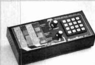
The **MM-2 Morsematic Keyer** represents the most sophisticated paddle keyer ever designed and features two powerful microcomputers. The Morsematic incorporates virtually all the features (except the preset and stepped variable speeds) of both the CK-2 and KT-2 shown above. In addition, the MM-2 offers an exclusive automatic beacon mode which is invaluable for meteor scatter, moonbounce scheduling, or beacon operation.
