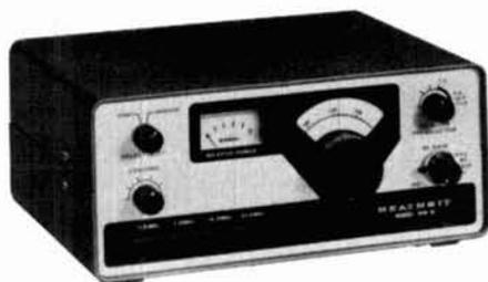
The HW-8 transceiver exhibits approximately 1500 Hz drift in transmit and receive frequency when the supply voltage varies over a range of 10 to 13.5 VDC. This results in CW chirp when using a poorly regulated supply, such as a weak, dry battery. Additionally, even with a well-regulated supply, the VFO dial calibration is in error on all but the 7 MHz band.
