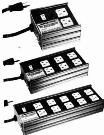
Designated "Surgefree," the new unit features all solid-state electronic circuitry. Compact in size, it can be plugged into any 120 VAC outlet to instantly sense and suppress destructive effects of high-voltage transient spikes and surges to sensitive electronic equipment. It is rated at 15 amps (1875 watt), 125 VAC, with a resettable circuit breaker that protects against accidental power overloads.
