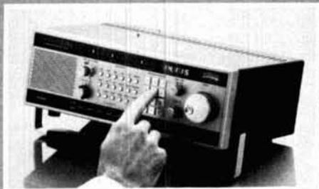
push buttons for selecting AM, LSB, USB, CW, or FM modes. The unit comes with a built-in telescoping antenna for portable use, and includes an SO-239 antenna connector for 50 ohm leads, and a screw connector for "High Z."
