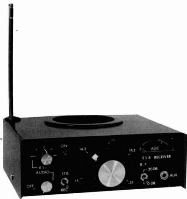
The completed receiver can be packaged to suit the builder. This 20-meter version features a signal-strength meter and a built-in voltage probe antenna system. The illuminated frequency pointer is an LED that has been filed to shape and polished.
