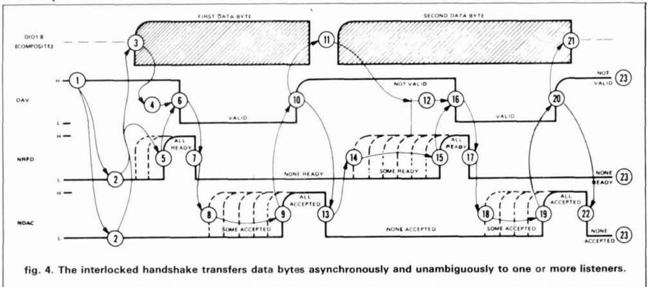
fig. 4. The interlocked handshake transfers data bytes asynchronously and unambiguously to one or more listeners.
