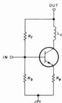
fig. 2. Simplified schematic of a 100 MHz bandwidth RF amplifier designed around the MWA module.
