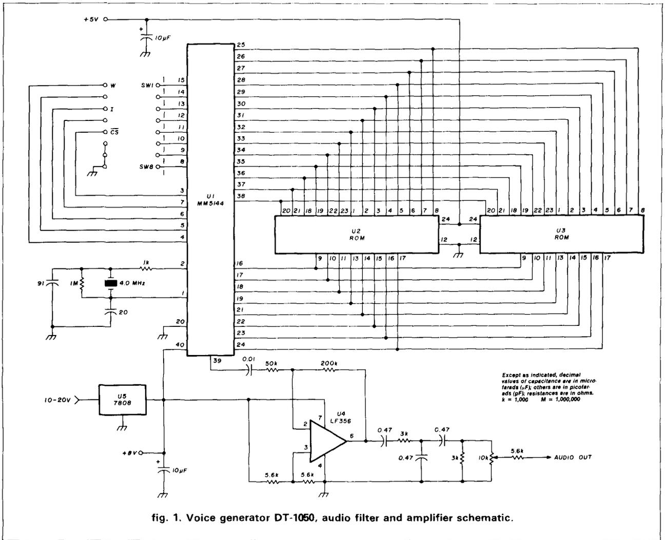
fig. 1. Voice generator DT-1050, audio filter and amplifier schematic.
