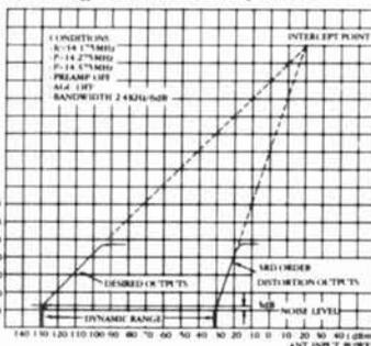
Feed Mixer), the IC-730 obtains a dynamic range of 100dB and an intercept point of 19.5dBm.
