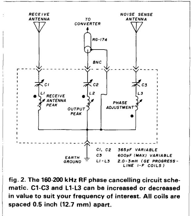
fig. 2. The 160-200 kHz RF phase cancelling circuit schematic. C1-C3 and L1-L3 can be increased or decreased in value to suit your frequency of interest. All coils are spaced 0.5 inch (12.7 mm) apart.
