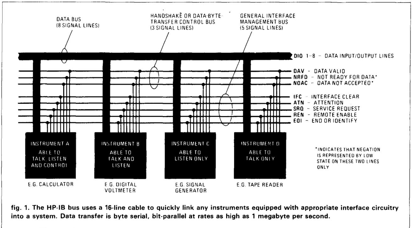
fig. 1. The HP-IB bus uses a 16-line cable to quickly link any instruments equipped with appropriate interface circuitry into a system. Data transfer is byte serial, bit-parallel at rates as high as 1 megabyte per second.
