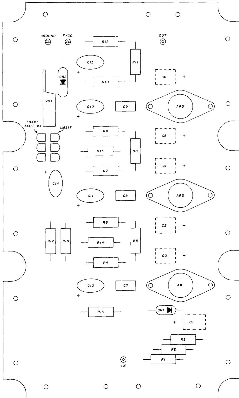
fig. 15. PC board component layout.
