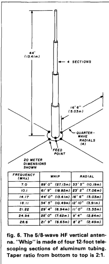
fig. 6. The 5/8-wave HF vertical antenna. "Whip" is made of four 12-foot telescoping sections of aluminum tubing. Taper ratio from bottom to top is 2:1.
