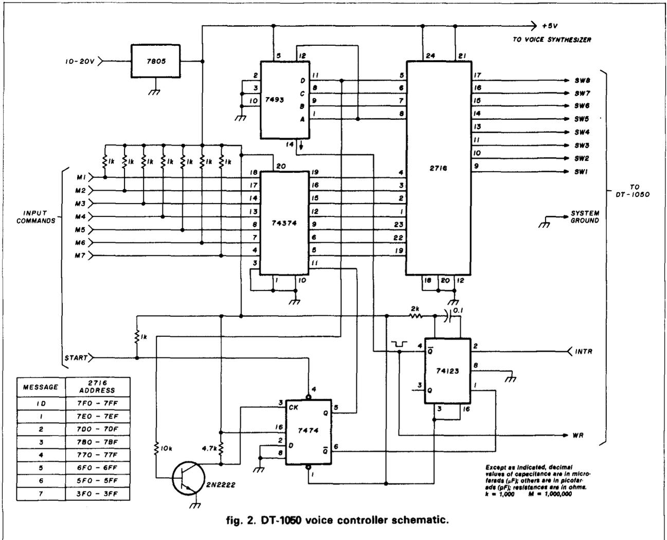
fig. 2. DT-1050 voice controller schematic.
