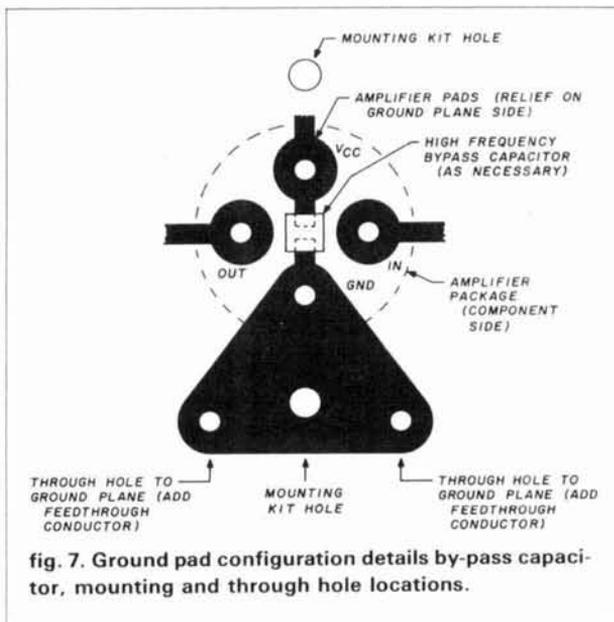
fig. 7. Ground pad configuration details by-pass capacitor, mounting and through hole locations.
