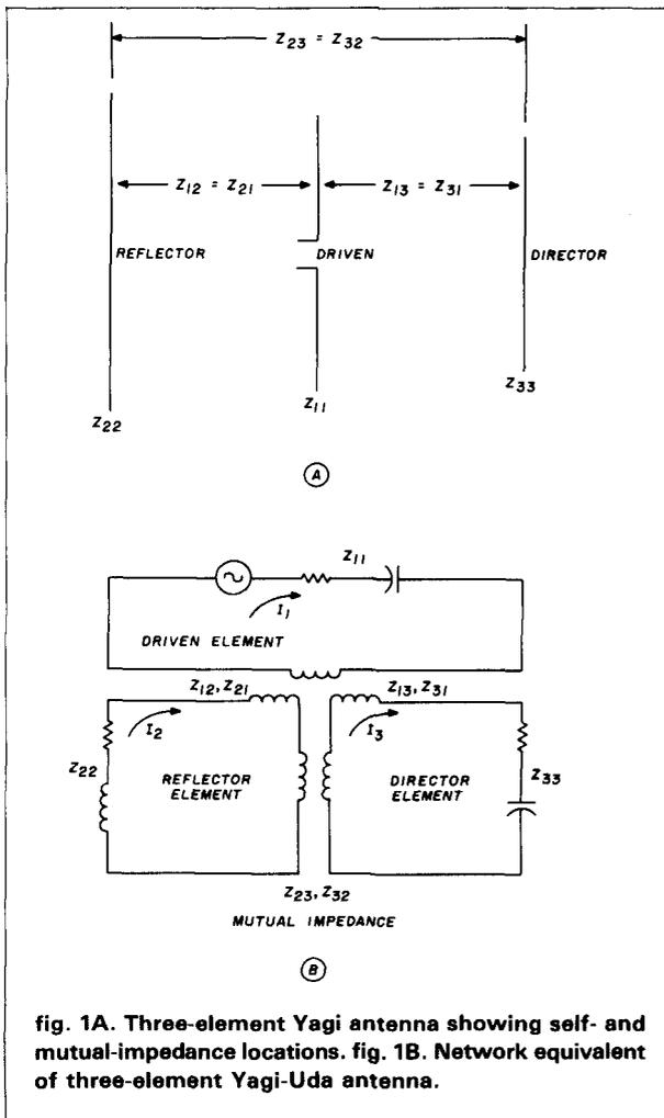
fig. 1A. Three-element Yagi antenna showing self- and mutual-impedance locations. fig. 1B. Network equivalent of three-element Yagi-Uda antenna.
