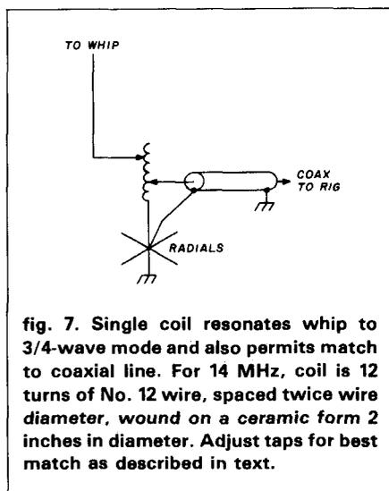
fig. 7. Single coil resonates whip to 3/4-wave mode and also permits match to coaxial line. For 14 MHz, coil is 12 turns of No. 12 wire, spaced twice wire diameter, wound on a ceramic form 2 inches in diameter. Adjust taps for best match as described in text.
