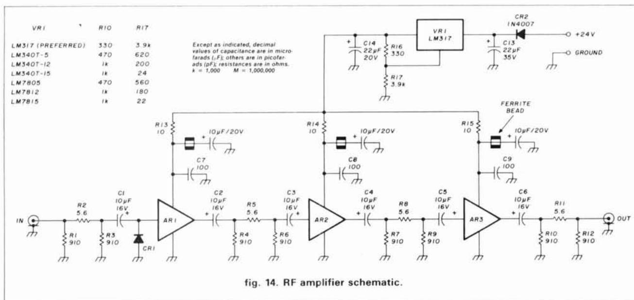
fig. 14. RF amplifier schematic.
