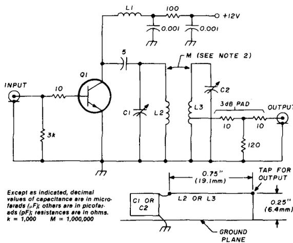
fig. 4. Frequency doubler: with a 190-220 MHz, 5-10 milliwatt input, a 380-440 MHz, 10-20 milliwatt output is produced.
