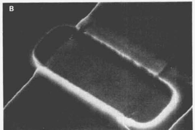
fig. 4. (A) shows static damage, magnified 7000 times, to a 3N157 MOSFET; (B) shows damage to an input pull-up resistor on a p-MOS character generator at 3000x magnification.
