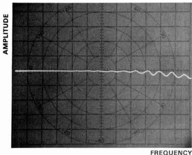
fig. 22. Test instrumentation actually introduces major ripple component.
