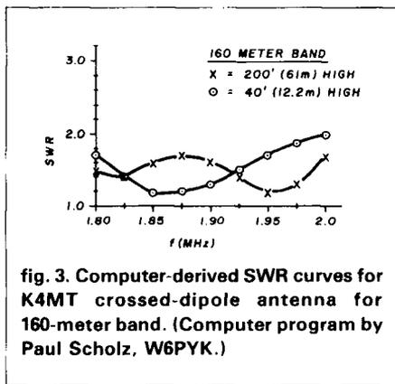
pedance and SWR readout. Two examples, given in fig. 3 and 4, show that even at low height, both the 80 and 160-meter designs exhibit a good match to a 50-ohm line; a better match, in fact, than if the antenna were suspended higher in the air.
