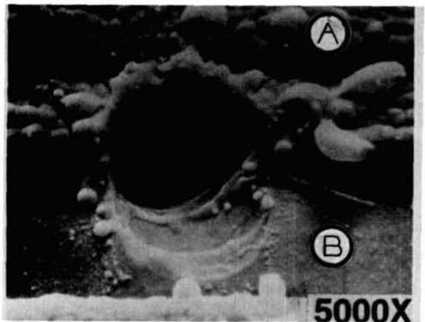
**fig. 1.** Enlarged, detailed views of a 6-micron (0.0002 inch) diameter hole created in aluminum metallization (A) and silicon dioxide substrate (B) by static electricity on an op amp integrated circuit.
