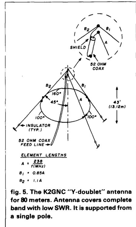
ductor. The wires form an angle of 45 degrees with respect to the 45-foot wooden support. The antenna wires also help guy the pole.
