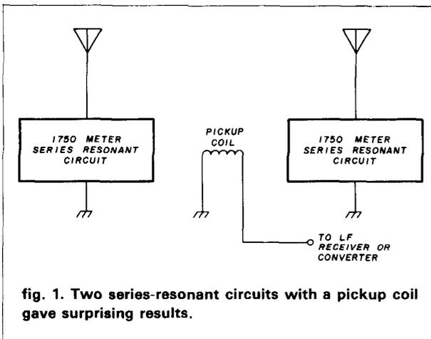
fig. 1. Two series-resonant circuits with a pickup coil gave surprising results.
