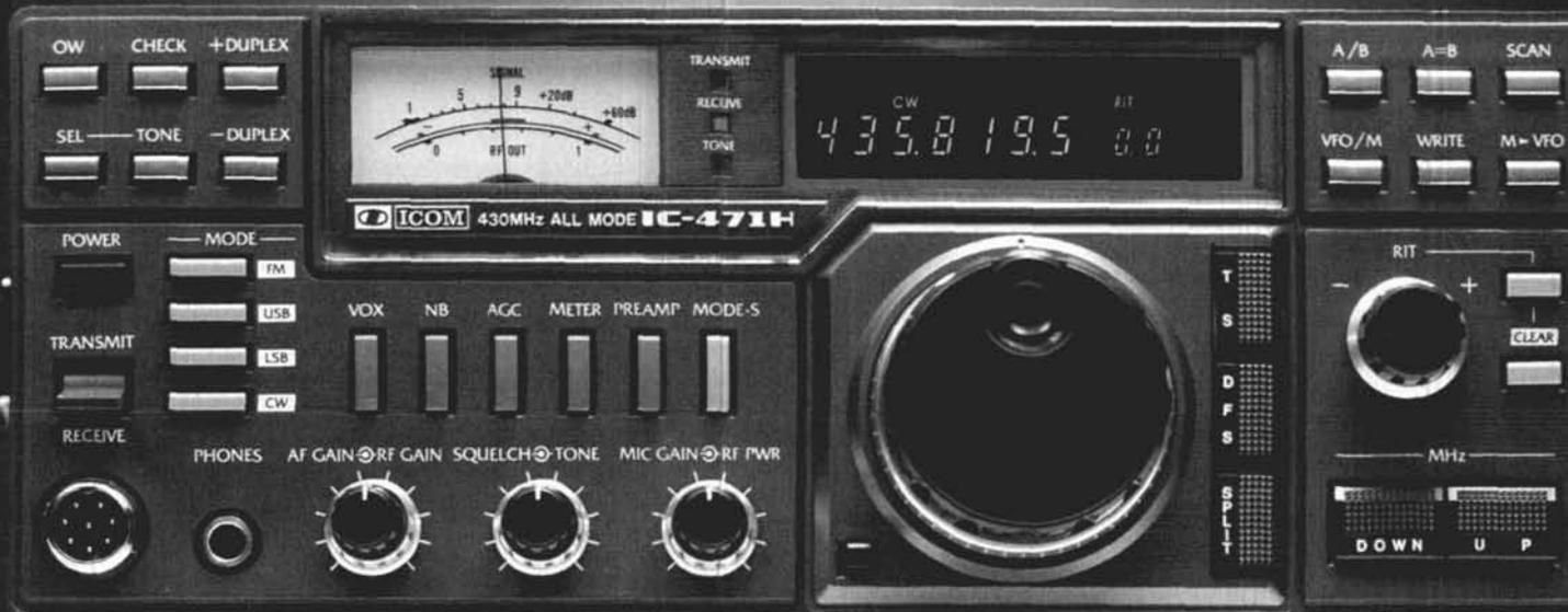
ICOM presents the IC-471H 430-450MHz base station transceiver with a 75-watt transmitter and high dynamic range, low noise receiver. With FM, CW or SSB modes plus the most advanced 10Hz PLL system, the IC-471H has features which give you maximum UHF operation.
