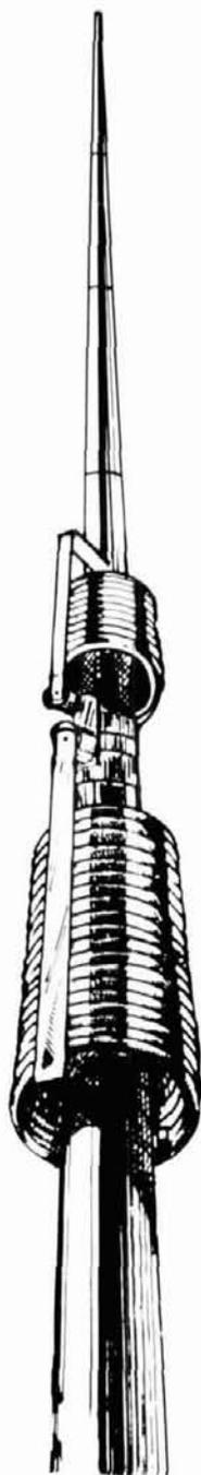
The HF2V is the perfect complement for the Ham who already has a beam antenna for 10-15-20 meters. Add 80 and 40 meters (160 meters with an optional resonator kit) with a trim-looking vertical that can be mounted almost anywhere.
