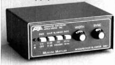
This extremely useful accessory is designed for direct insertion between your receiver (or transceiver) and the antenna. It is both MORE EFFECTIVE than I.F. type blankers and requires NO MODIFICATIONS to your receiver! The unit operates from a 13 VDC  $\pm$  2 VDC power source at less than 575 mA. (AEA AC wall unit AC-1 will operate the blanker.)
