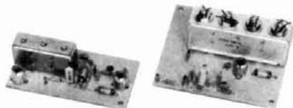
Our lab has developed a new line of low-noise receiver preamps with helical resonator filters built in. The combination of a low noise amplifier and the sharp selectivity of a 3 or 4 section helical resonator provides increased sensitivity while reducing intermod and cross-band interference in critical applications. See selectivity curves at right. Gain = approx. 12 dB.
