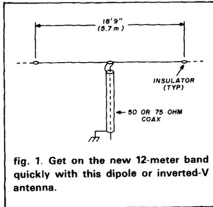
fig. 1. Get on the new 12-meter band quickly with this dipole or inverted-V antenna.
