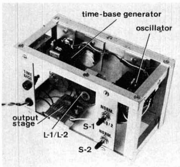
Inside view of the IF sweep generator. Circuit simplicity and ordinary components provide a versatile test instrument.
