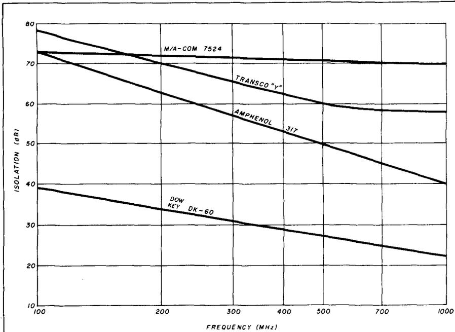
fig. 3. Typical values of isolation on some of the more popular T/R relays used by Amateurs.
