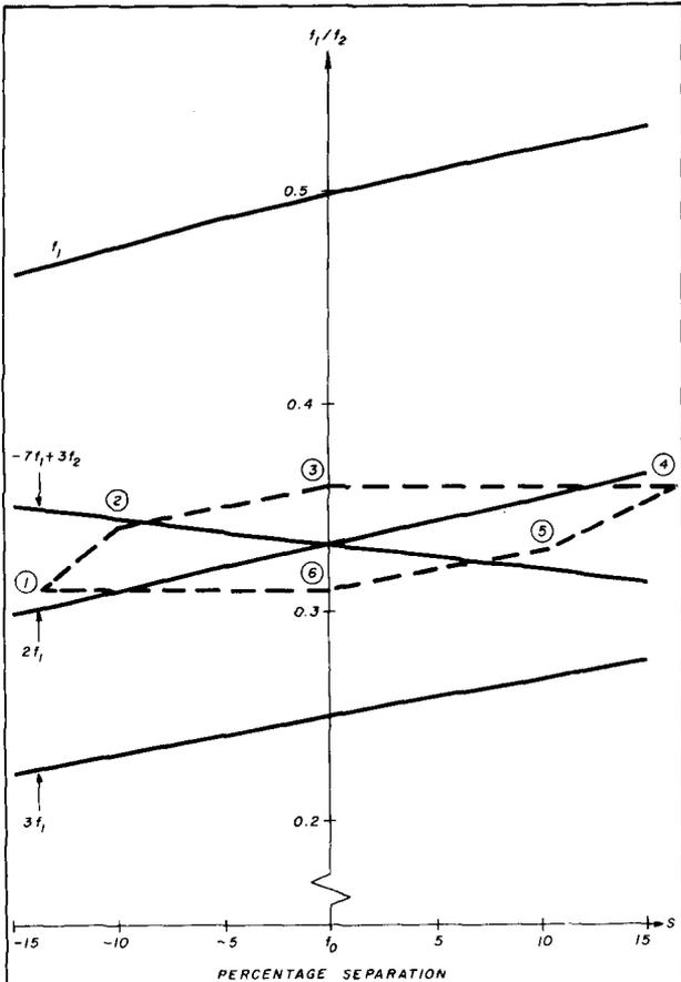
fig. 2. Spur chart for conversion of bands of frequencies —  $f_0 = f_2 + f_1$ . The circled numbers (1-6) are those referred to in the text and listed in table 2.
