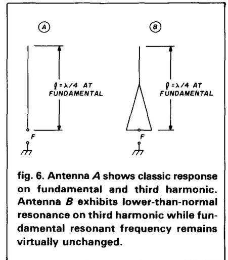
fig. 6. Antenna **A** shows classic response on fundamental and third harmonic. Antenna **B** exhibits lower-than-normal resonance on third harmonic while fundamental resonant frequency remains virtually unchanged.
