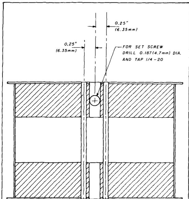
2.5 x 11.5 inch (6.35 x 29.2 cm) of 0.010 to 0.012 inch (0.25 to 0.3 mm) thick aluminum sheet (used printing plate). Position end disks on 0.25 inch (6.3 mm) rod for alignment. Wrap around end disks, cemented with epoxy (including overlap). Secure with sufficient rubber bands until set. Align carefully so aluminum sheet does not overhang disks.
