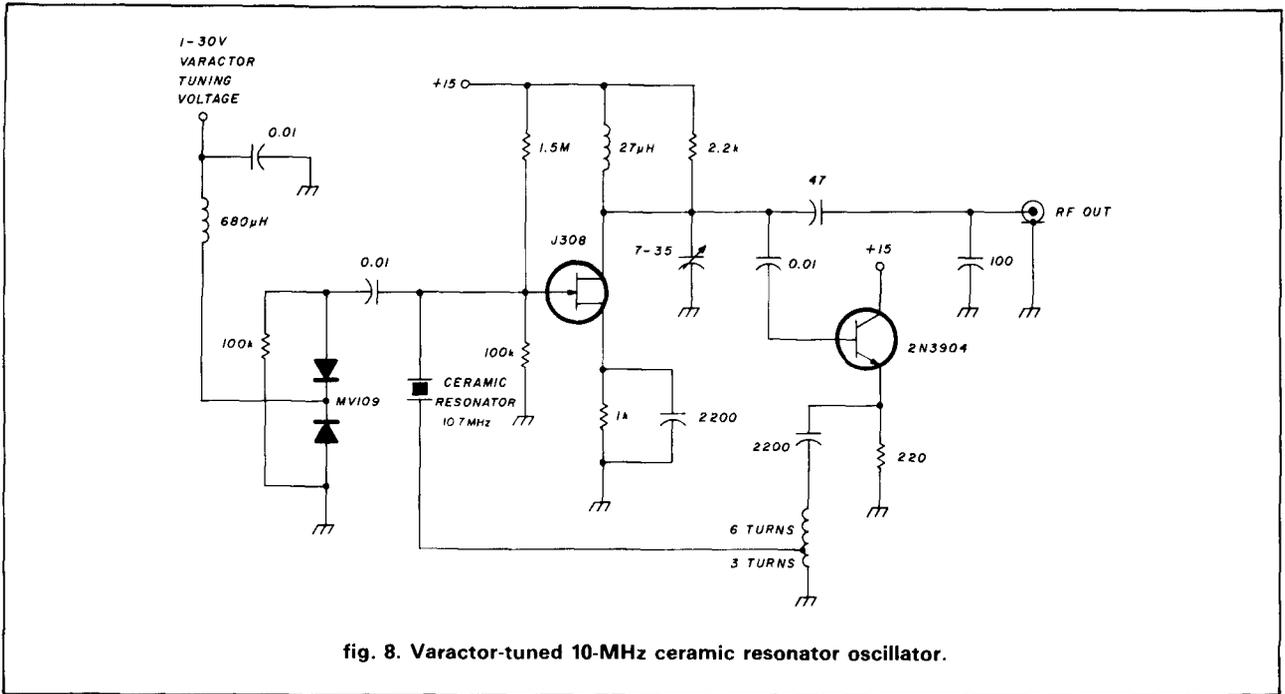
fig. 8. Varactor-tuned 10-MHz ceramic resonator oscillator.
