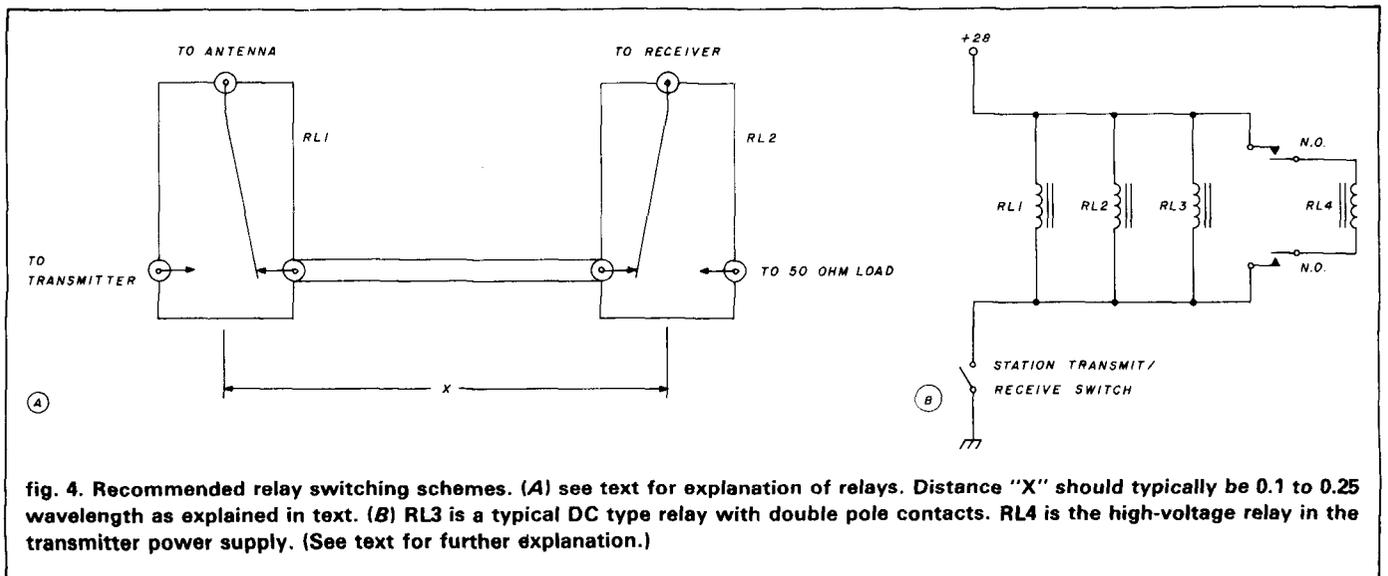
fig. 4. Recommended relay switching schemes. (A) see text for explanation of relays. Distance "X" should typically be 0.1 to 0.25 wavelength as explained in text. (B) RL3 is a typical DC type relay with double pole contacts. RL4 is the high-voltage relay in the transmitter power supply. (See text for further explanation.)
