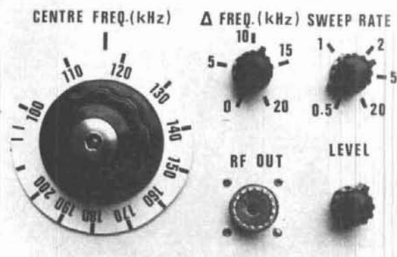
IF sweep generator has a frequency range of 1:2 with excellent linearity.
