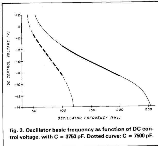
fig. 2. Oscillator basic frequency as function of DC control voltage, with C = 3750 pF. Dotted curve: C = 7500 pF.
