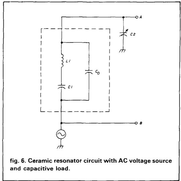
fig. 6. Ceramic resonator circuit with AC voltage source and capacitive load.
