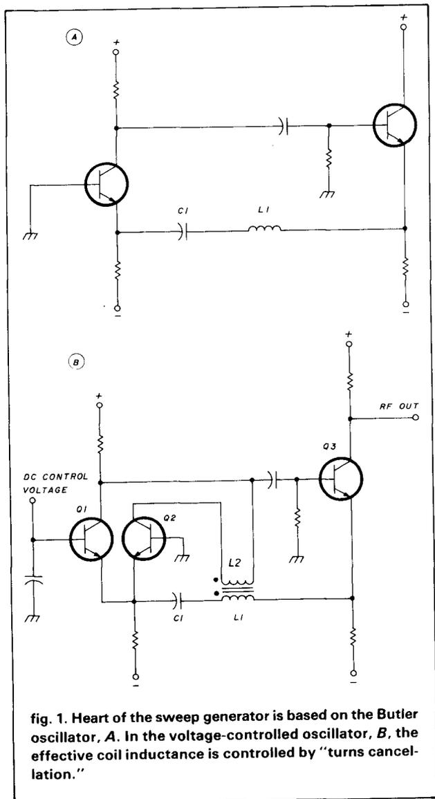
fig. 1. Heart of the sweep generator is based on the Butler oscillator, A. In the voltage-controlled oscillator, B, the effective coil inductance is controlled by "turns cancellation."
