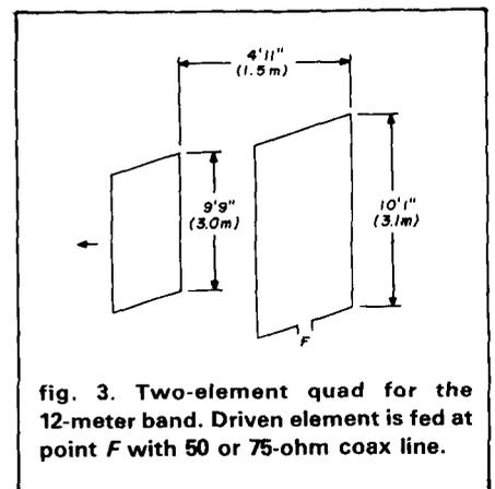
fig. 3. Two-element quad for the 12-meter band. Driven element is fed at point F with 50 or 75-ohm coax line.
