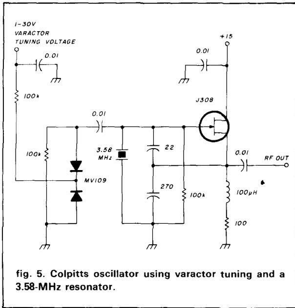
fig. 5. Colpitts oscillator using varactor tuning and a 3.58-MHz resonator.
