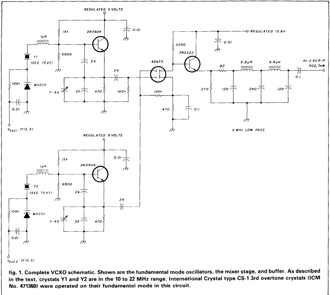
fig. 1. Complete VCXO schematic. Shown are the fundamental mode oscillators, the mixer stage, and buffer. As described in the text, crystals Y1 and Y2 are in the 10 to 22 MHz range. International Crystal type CS-1 3rd overtone crystals (ICM No. 471360) were operated on their fundamental mode in this circuit.
