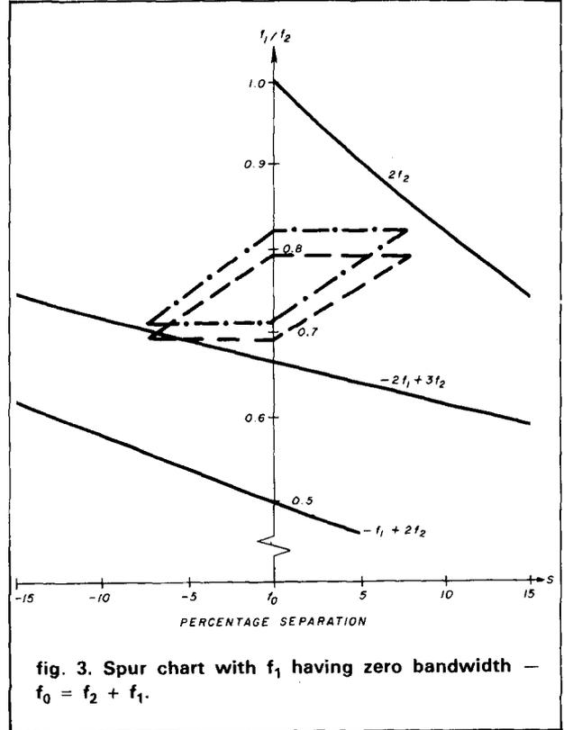
fig. 3. Spur chart with  $f_1$  having zero bandwidth —  $f_0 = f_2 + f_1$ .
