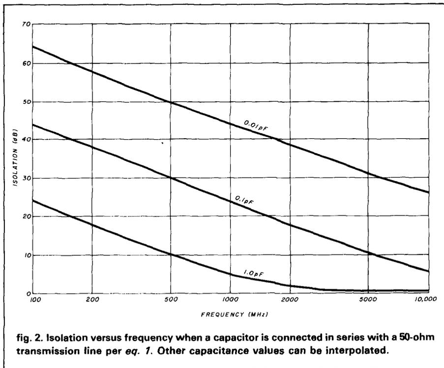
fig. 2. Isolation versus frequency when a capacitor is connected in series with a 50-ohm transmission line per eq. 1. Other capacitance values can be interpolated.
