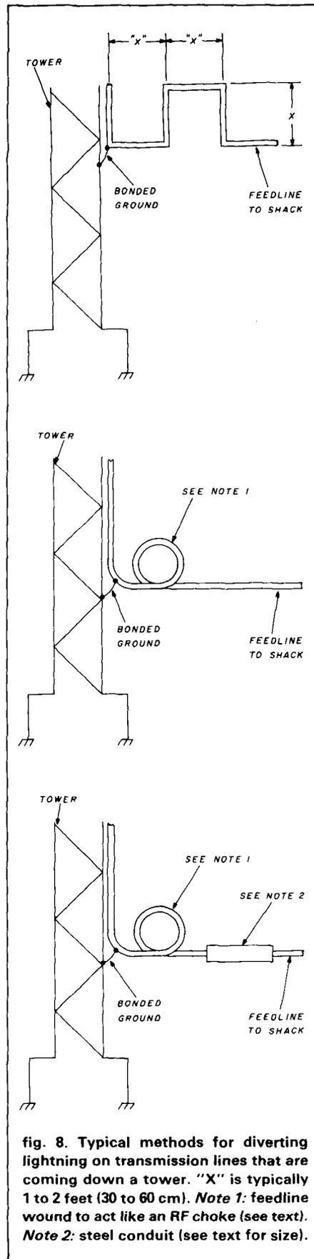
fig. 8. Typical methods for diverting lightning on transmission lines that are coming down a tower. "X" is typically 1 to 2 feet (30 to 60 cm). Note 1: feedline wound to act like an RF choke (see text). Note 2: steel conduit (see text for size).
