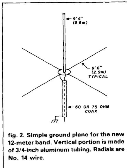
fig. 2. Simple ground plane for the new 12-meter band. Vertical portion is made of 3/4-inch aluminum tubing. Radials are No. 14 wire.
