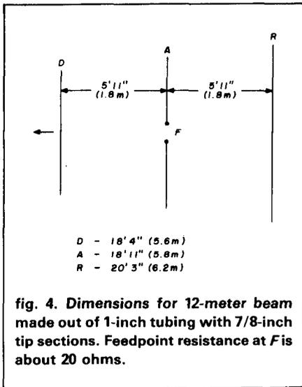
fig. 4. Dimensions for 12-meter beam made out of 1-inch tubing with 7/8-inch tip sections. Feedpoint resistance at F is about 20 ohms.
