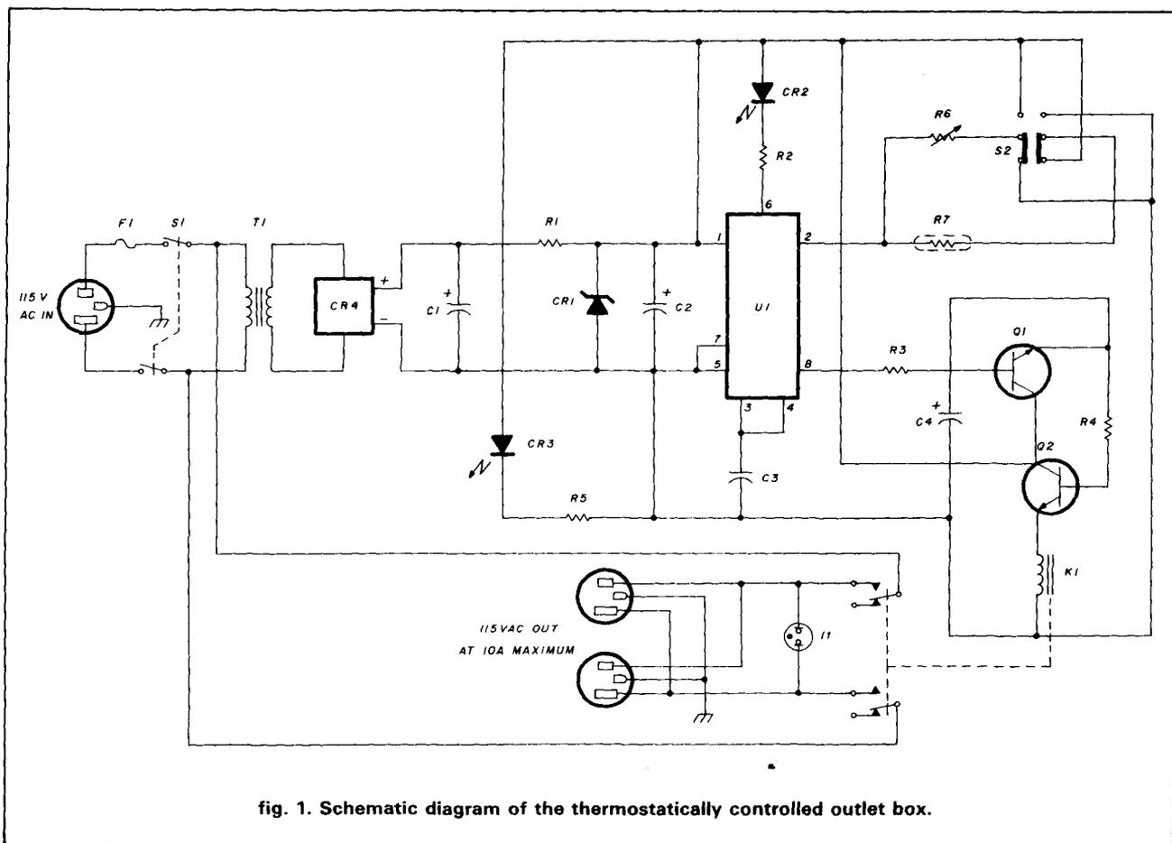
fig. 1. Schematic diagram of the thermostatically controlled outlet box.
