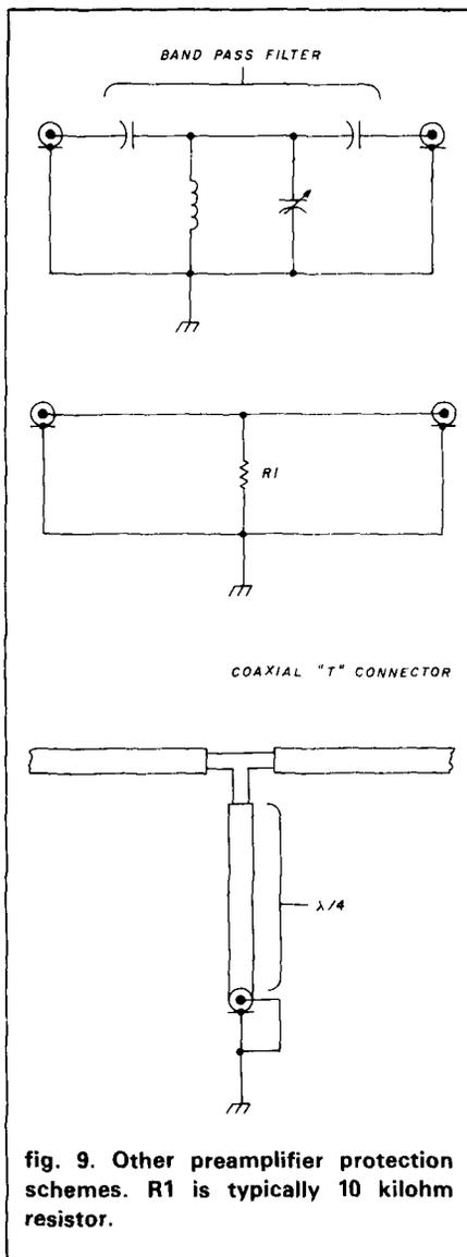
fig. 9. Other preamplifier protection schemes. R1 is typically 10 kilohm resistor.
