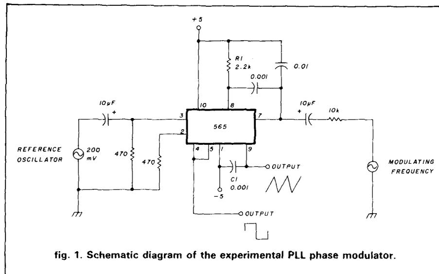
fig. 1. Schematic diagram of the experimental PLL phase modulator.
