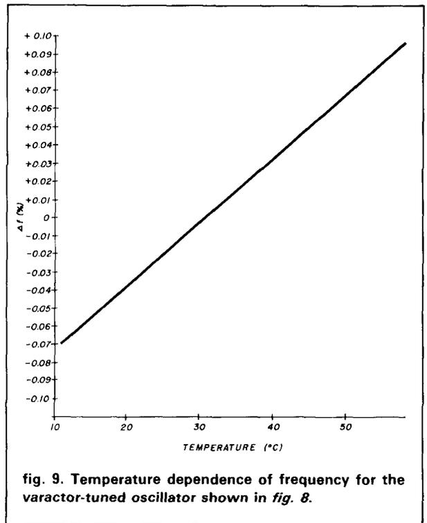
fig. 9. Temperature dependence of frequency for the varactor-tuned oscillator shown in fig. 8.
