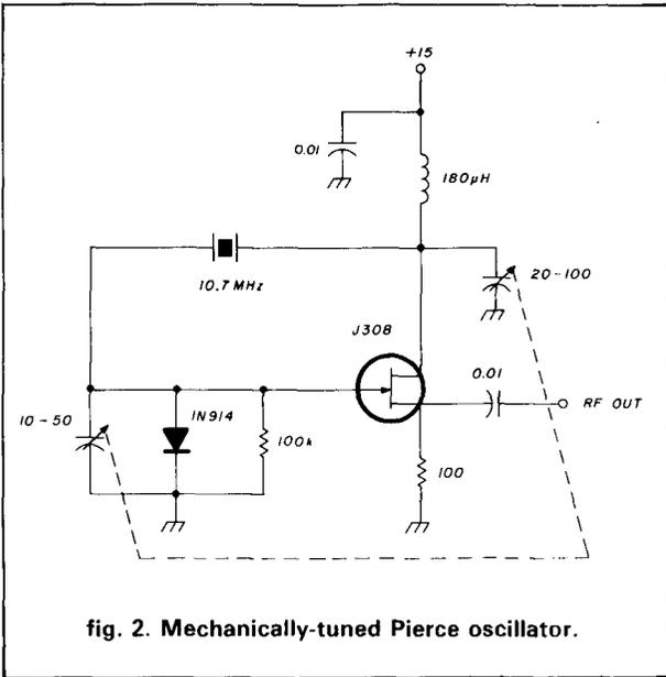
fig. 2. Mechanically-tuned Pierce oscillator.
