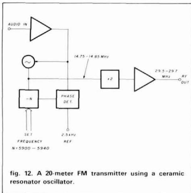
fig. 12. A 20-meter FM transmitter using a ceramic resonator oscillator.
