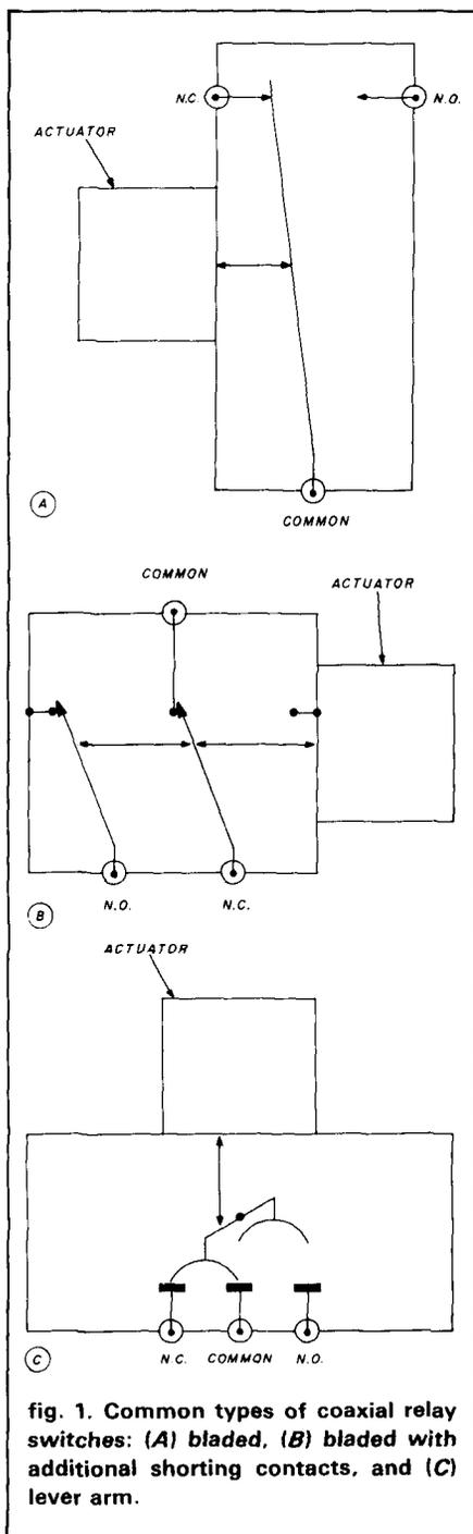
fig. 1. Common types of coaxial relay switches: (A) bladed, (B) bladed with additional shunting contacts, and (C) lever arm.
