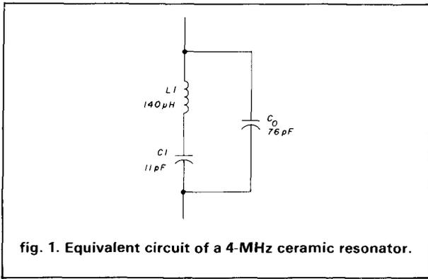
fig. 1. Equivalent circuit of a 4-MHz ceramic resonator.
