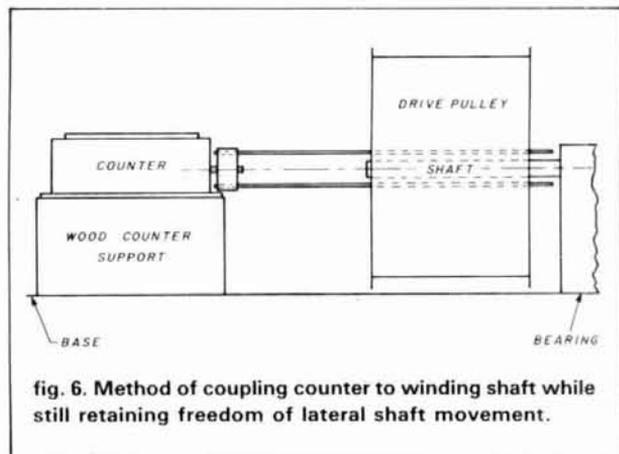
my opinion the top of the shaft should be moving away from you when you stand in front of the winder; this facilitates inserting insulation papers and observing the wire as it winds on.
