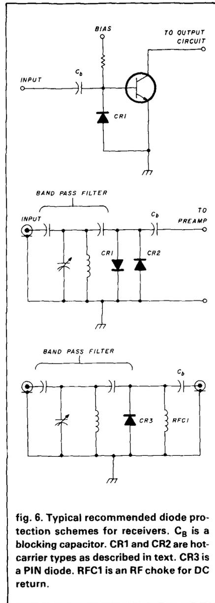
fig. 6. Typical recommended diode protection schemes for receivers.  $C_b$  is a blocking capacitor. CR1 and CR2 are hot-carrier types as described in text. CR3 is a PIN diode. RFC1 is an RF choke for DC return.
