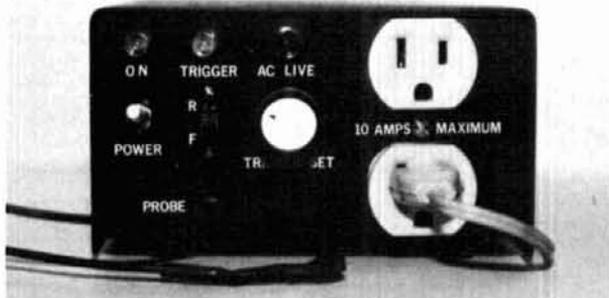
fig. 3. View of the front panel. Coiled black wire contains thermistor R7 (covered with heatshrink tubing) at one end.
