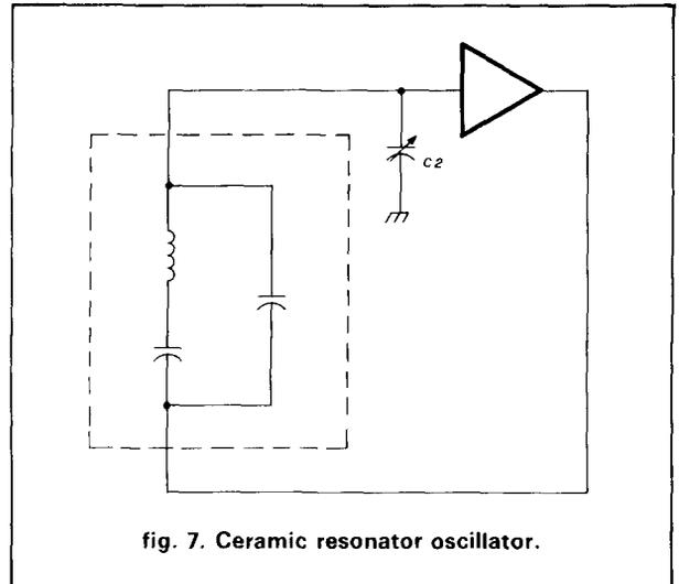
fig. 7. Ceramic resonator oscillator.
