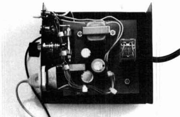
fig. 2. Internal view, with top cover removed. F1, T1, and K1 are mounted near the top of the board. U2 is barely visible beneath the wiring at the lower left corner of the board.
