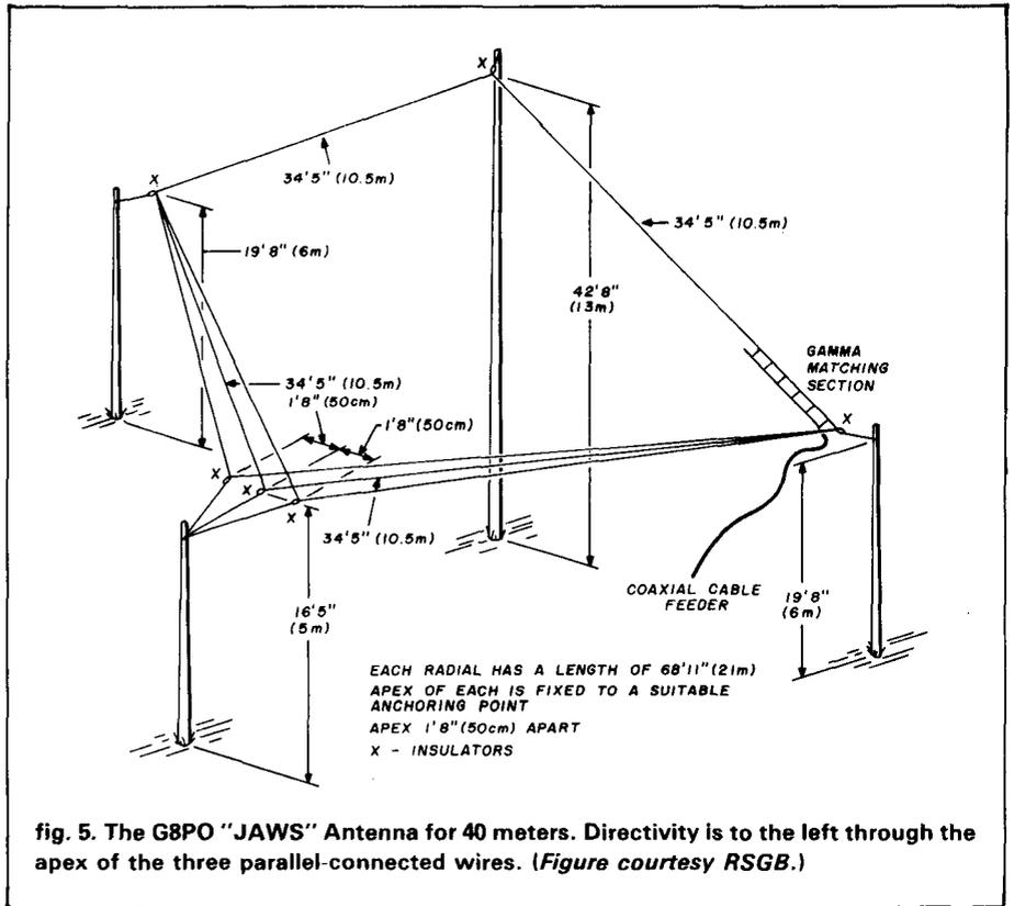
fig. 5. The G8PO "JAWS" Antenna for 40 meters. Directivity is to the left through the apex of the three parallel-connected wires. (Figure courtesy RSGB.)
