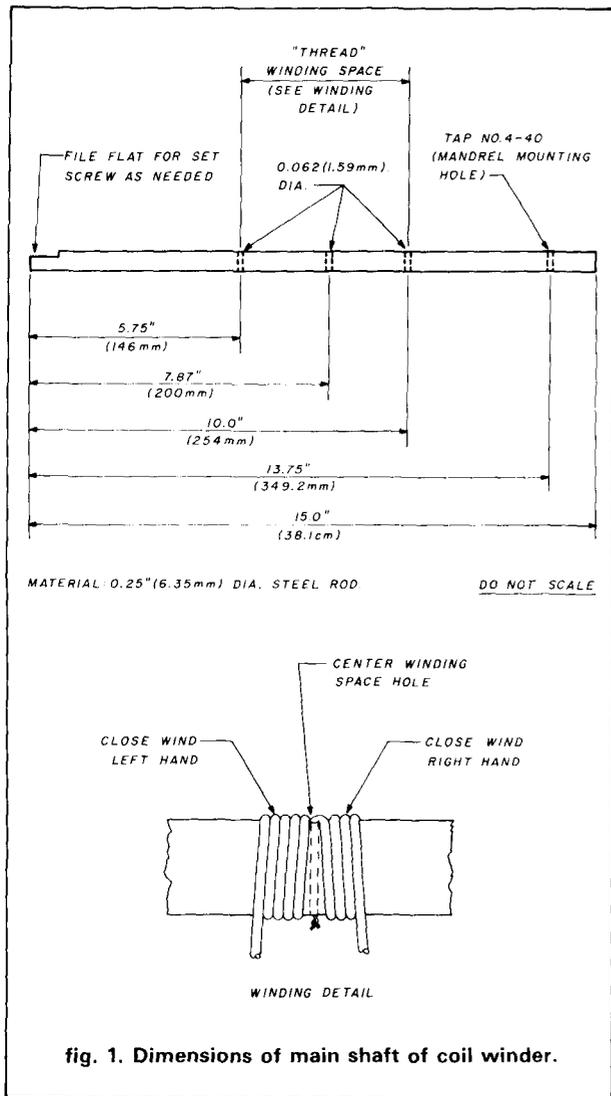
fig. 1. Dimensions of main shaft of coil winder.
