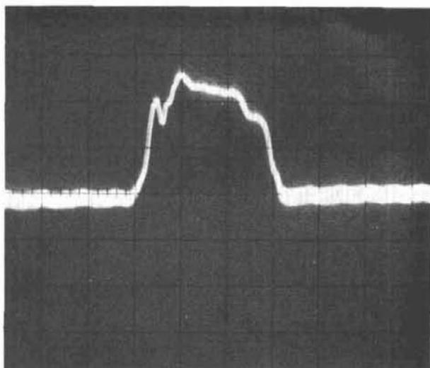
fig. 7. *Top*: Response of IF amplifier with 9 MHz crystal filter in HF transceiver. Sweep rate 4 Hz. *Bottom*: poorly matched mechanical bandfilter in 455 kHz IF amplifier (Collins F455-J-31). Sweep rate 4 Hz.
