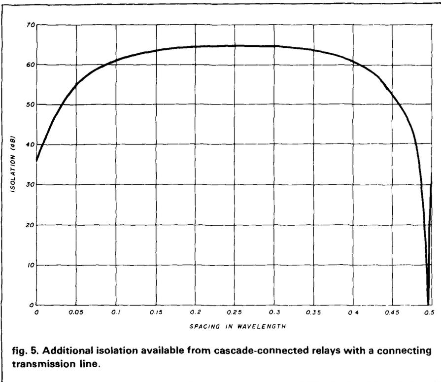
fig. 5. Additional isolation available from cascade-connected relays with a connecting transmission line.
