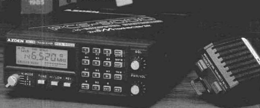
**UNPRECEDENTED WIDE FREQUENCY RANGE:** Covers 140,000-153,000 MHz in steps that can be set to any multiple of 5 kHz up to 50 kHz.
