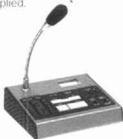
**MC-85** (8-pin) Multi-function desk-top microphone (8-pin) 700  $\Omega$  unidirectional electret condenser mic. Built-in audio level compensation with output and tone control, meter, and UP/DOWN switch. Selector switch for up to three transceivers. (Additional 4, 6, or 8-pin cables optional.)
