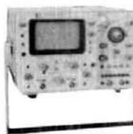
Portable dual-trace DC to 75 MHz scope with 6x10 cm display and <4.7 nS risetime. Deflection 10 mv - 5 V/div in 9 ranges. Sweep 0.1 uS - 2 S/div in 23 ranges; delay 0.1 uS - 0.2 S/div. 7.8 x 12.8 x 16, 32 lbs sh. HP-quality at import price.
