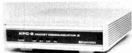
Power supply, connectors, and cables are provided with the KPC-2, but the user must supply the transceiver mic jack and the computer RS232/TTL connector.
