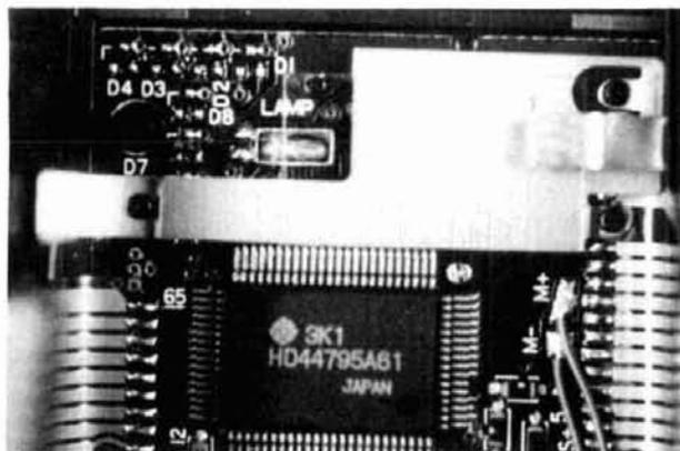
Fig. 3. Initialization diodes can be located at positions D1-D4, which are found at the top left corner of the microprocessor circuit board. The factory diodes are surface mounted on the triangular pads at D2 and D3 for the IC-02, and at D1 and D2 for the IC-04. The IC-02 is modified by simply removing the diode at position D2. To modify the IC-04, remove the diode at position D2 and replace it with a 1N914-type connected from the top pad (anode) to the lower right pad (cathode).
