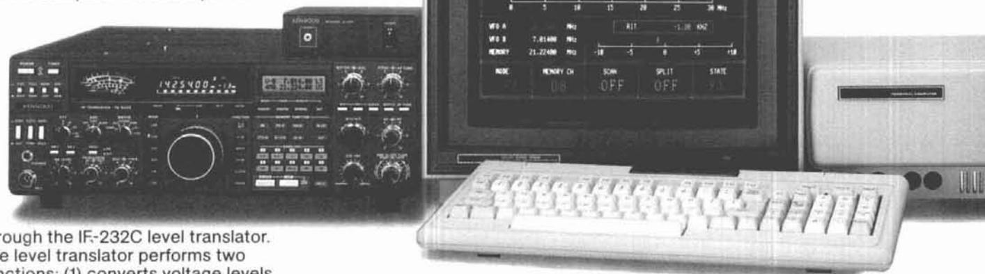
through the IF-232C level translator. The level translator performs two functions: (1) converts voltage levels from the RS-232C port to the TTL levels in the transceiver, (2) and acts as a noise suppressor. A complete interface "kit" would include the appropriate computer interface units (IF-10A, IF-10B, or IC-10) and the IF-232C level translator.
