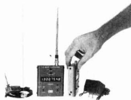
of even a weak signal (i.e., for a counter), the count stabilizes and you know the unit's working. In one quick test, the counter performed faultlessly on a handheld unit pushing 500 mW into a rubber duck over distances up to about 50 feet through an exterior (wooden) wall.
