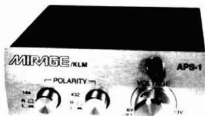
The APS-1 may be powered by the power adaptor (included) or may alternately be powered from a vehicle or other 13-17 VDC source.
