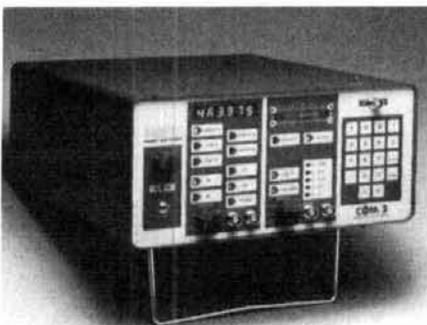
Monitor, designed for analyzing and testing transceivers in the 100-kHz to 1000-MHz range, features a programmable microprocessor memory that stores and recalls up to ten commonly used test set-ups. It covers every band and frequency, and i-f parameters of 100 kHz to 1000 MHz in 1 kHz steps. The keyboard features programmable offset keys that simplify frequency entry for duplex or repeater radios, and incremental step keys to facilitate receiver testing.
