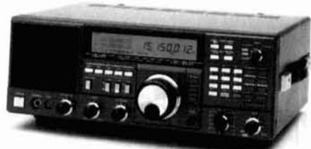
**World-class HF receiver.** The FRG-8800's perfect for keeping up with the world. Continuous coverage from 150 KHz to 30 MHz. Expanded coverage with optional 118-174 MHz VHF converter. USB, LSB, CW wide/narrow, AM wide/narrow, FM. 12 memories. Also programmable scanning routines. Keyboard frequency entry. LCD display. SINPO signal graph. Computer interface capability. Two 24-hour clocks. Recording functions. Much more.
