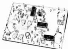
**COR-3 REPEATER CONTROL-ER** kit. Features adjustable tail & time-out timers, solid-state relay, courtesy beep, and local speaker amplifier. ....\$49
