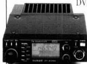
**7 Mobiles you can take on foot.** Our FT-290R Mark II Series (2-meter, 430-450 MHz, and 6-meter models) come standard as mobiles. But remove the heat sink and snap-on the optional battery pack, and you're ready to take your operation on foot! Mobile operation: 25 watts output (10 watts, 6 meters). Battery pack: 2.5 watts output. With SSB, CW and FM. 10 memories. Dual VFOs. LCD display. Offset tuning. Relative power-output/S meter. More.
