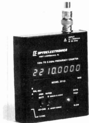
Input sensitivity is less than 10 mV from 10 Hz to 2 GHz; 3 mV is typical. Accuracy is 1 PPM with temperature compensated crystal oscillators. Resolution is 1 Hz below and 100 Hz above 12 MHz. A full 16-hour recharge yields 2 hours of battery operation. Use an AC adapter/charger to operate when recharging.
