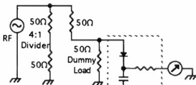
Fig. 3: Higher Power Measurement Using A 4:1 Power Divider
