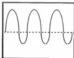
Figure 2: Output waveform of a bipolar oscillator
