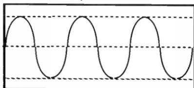
Figure 4: Output waveform of tuned-emitter oscillator
