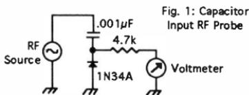
Fig. 1: Capacitor Input RF Probe
