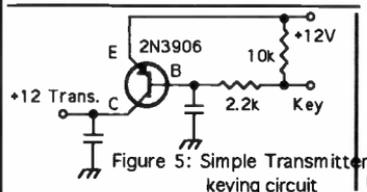
Figure 5: Simple Transmitter keying circuit
