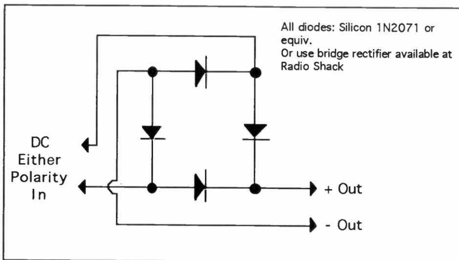
If you like to work on DC stuff, here is a little device that might save a power supply for you. It can be easy to get the positive and negative leads mixed up while working on a radio on your crowded work bench.
