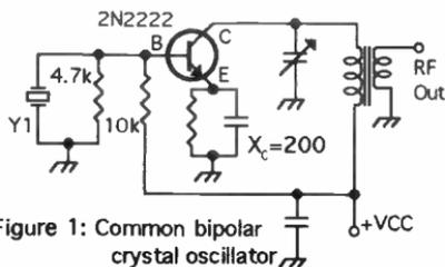
Figure 1: Common bipolar crystal oscillator
