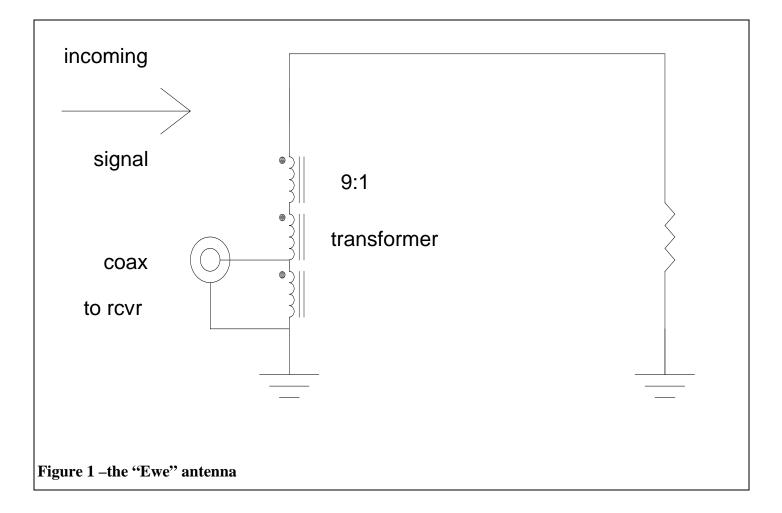
For the amateur bands, the "Ewe" is a length of wire about 10 feet high and up to 60 feet long. It has two downleads, one to the receiver through a 9:1 matching transformer to ground, and one at the opposite end which is terminated to ground through a resistor (see Figure 1) which is adjusted
