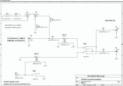
The FCA-1 allows the 60 m feedline going to the amplifier base of the farther antenna to be used as an antenna itself.
