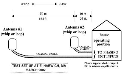
Field-site antenna amplifier boxes were TMB-1's (reference 1) . These can be used in one configuration for active whip operation (I used a 1.83 m / 6 ft. telescoping rod) and in another configuration for broadband loop operation (using, in this case, a 2 m per side square loop of wire mounted in a vertical plane).
