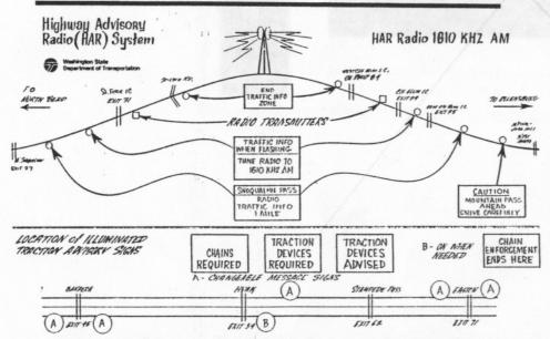
This is a diagram of the TIS system used by the Washington Dept of Transportation along I-90 across Snoqualmie Pass. They added a transmitter at the top of the pass since this drawing was produced. Note how the transmitters and signs are integrated together.
