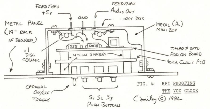
FIG. 4 RFI PROOFING THE VOX CLOCK
