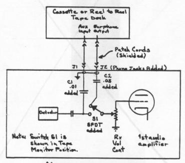
Modified Receiver Wiring
