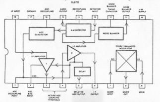
Sounds like the answer to a receiver designer's prayer, and to a large degree it is. The SL6700 was featured in a receiver description article in  $\frac{QST}{100}$  of April 1981, and I took the circuit in that article, and combined it with a circuit described in the IC's spec sheet to come up with the wiring below:  $5_{\rm w}F$
