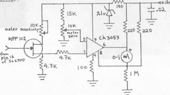
The "meter zero" trimpot is used to set the meter at zero when no signal is coming in, while the "meter sensitivity" trimpot sets the meter at its maximum reading when you local is tuned in.
