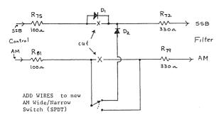
The switch can be installed in a number of spots (the wires need not be shielded as they only carry a small DC switching voltage) such as:
