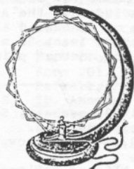
1926 loop antenna made by Eclipse Radio Laboratories; a basketweave antenna could be rotated easily on its pivot.
