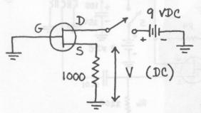
Ql and Q2 should be matched pairs of MPF102's, and Q3 amd Q4 should be matched pairs of MPF102's. It is not necessary or desirable that all 4 FET's be matched. The best way I know to match FET's is due to Kolb and Sanserino, and is shown at left. Measure the DC voltage across a 1000 ohm source resistor as shown, and select pairs of FET's with measured
