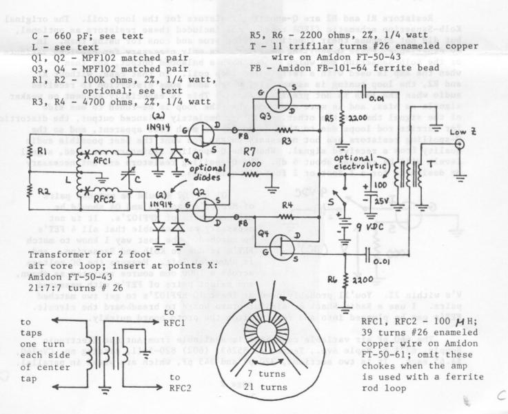
Another major difference between my amp and all previous variants of the Kolb-Sanserino amp are the 100 micro-Henry chokes RFCl and RFC2. The chokes are not necessary or desirable when the amp is used with a ferrite rod loop; they should be omitted in that case. The chokes are necessary to eliminate 2nd order IMD products due to SW signals when the amp is used with 1 foot or 2 foot air core loops as described below.
