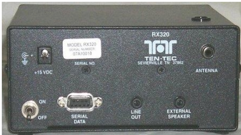
Figure 1 -- rear view of RX-320
