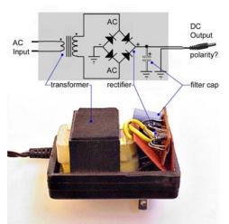
through a solid-state "bridge" (four diodes) or "full-wave" (two diodes) rectifier to be converted to DC. This is usually followed by a single filter capacitor. The power is then piped out through twin wires of appropriate size to carry the current at the designed power level. It is my understanding that some very inexpensive wall warts do not contain even rudimentary filter capacitors. Avoid these, if possible.
