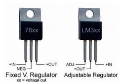
Bill recommended using two families of small integrated circuit voltage regulators for our more common applications: the 78xx family of fixed voltage regulators and the LM3xx family of adjustable regulators. Both of these families are popular in commercial and hobby applications and are manufactured in great numbers; hence, they are all quite commonly available and very low cost. A grid of reference information for each family which follows:
