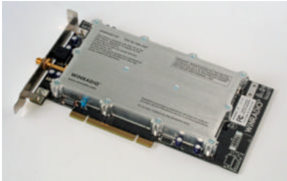
Fig. 2 The G3 series of SDRs from Australian company WinRADIo is available either as external boxes or as PCI cards that plug into one of the expansion slots inside the PC.
