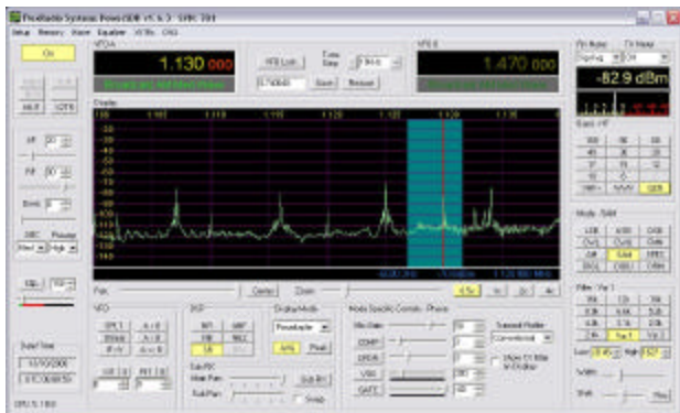
Fig. 3 Every SDR provides a real-time bandscope to display a range of frequencies around the one that you're tuned to. You can see here that there are signals visible on every European and American channel.
