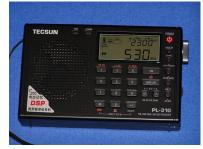
advantages of the PL-310, plus complete freedom from the one disadvantage plaguing all the DSP pocket radios produced thus far... the irritating "soft mute" function, a major drawback for weak-signal AM-DXers.
