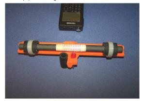
and secure your loopstick on the completed plastic frame, using the suggested rubber shock mounts to protect the ferrite bar.
