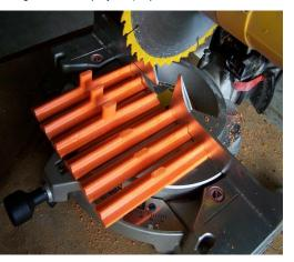
least 3" of space between the holes, so that the short frame sections of 1.5" x 2" can eventually be cut with the miter saw (see photo below).
