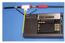
In general the system worked very well; although Lincoln City's location to the southwest of Portland, Oregon (and Seattle, Washington) meant that the 3' loop encountered some domestic splatter from the back side on certain frequencies as it chased DU's to the southwest, due to its figure-8 reception pattern. The 1 kHz DSP selectivity of the Tecsun PL-380 tended to minimize this
