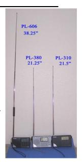
although it is very important to ensure a solid electrical connection (inside the plastic clamp) between the stock whip antenna tip and the metal base tip of the extender antenna. When the PL-606 has this accessory fully extended (photo at right), the composite whip antenna is much longer than those of either the PL-380 or PL-310 models—resulting in superior reception of fringe FM.
