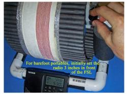
2) For a "barefoot" portable radio (without any transplanted loopstick), initially place the portable radio so that the radio's loopstick is about 3" (75 mm) in front of the FSL coil (see photo above right). For radios with a transplanted 7.5" loopstick, initially place the radio about 7" (18 cm) in front of the FSL coil.
