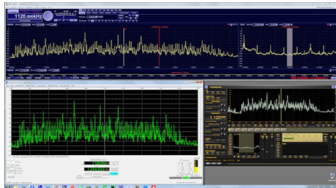
Figure 1--- All SDRs present a visual interface with spectrum displays and operating controls on screen. These are the dedicated software applications for three leading SDRs. All are tuned to 1120 kHz and are displaying the whole of the MW band. Across the top is the Winradio Excalibur Pro, below it on the left is the RFspace NetSDR, and bottom right is the Microtelecom Perseus.
