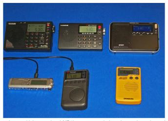
For the first time in any competitive radio review, multiple test signal MP3's were recorded to give each reader a chance to listen to accurate evidence of the relative performance of each model in important categories. These categories were MW sensitivity, MW selectivity, FM sensitivity, Shortwave sensitivity and Weather Band sensitivity
