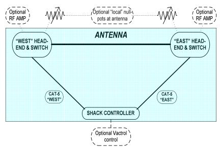
The antenna head-ends can include local null-pots for those of us who use "set-and-forget" nulling. For remote control of the null, Vactrols may be built in. The head-ends can also accommodate individual RF amplifiers at both ends. (Quiet 12-volt dc amplifier power is delivered via the 4<sup>th</sup> Cat-5 Pair.)
