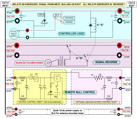
CONTROL LOGIC: The 12vdc control circuit to both Pair 3's drives the slave relays at each head-end. "K-S" in this drawing switches the signal path in concert with the relay switching at the head-ends. That's all you need for a basic reverser. Our system is set up so that when power is off, relaxed relays make "West" the default direction. When the reverser is enabled, all relays operate in tandem (combined current draw 160ma).
