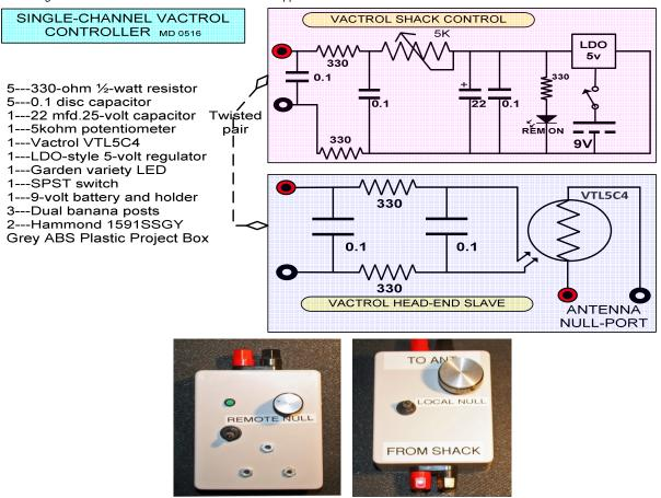
This controller provides "single-ended" antenna control and is usually all you need... unless you want to flip the antenna without major rewiring. To turn the unidirectional antenna into a reversible array we add some simple relay switching.
