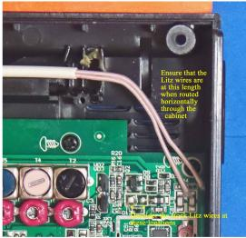
20) Refer to the close up photo above. Using a low heat (25w) pencil-type soldering iron, remove the two stock Litz wire leads at the positions shown, taking care not to use excessive heat, or touch the adjacent components. Ensure that the new Litz wire leads are at the length shown when the leads are in a horizontal position throughout the cabinet, and cut them to this length if they are not.
