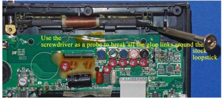
10) Refer to the photo above. Using a flat Jeweler's screwdriver with a 1/16" blade, carefully probe around all four sides of the stock loopstick to break all of the glue bonds. Work slowly and carefully around the perimeter of the ferrite rod, including the plastic covers on each end. Once most of the glue bonds have been broken the ferrite rod will begin to shift around as you break up the few remaining bonds, but until this point work slowly and patiently to break up the glue.
