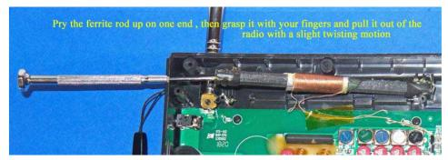
11) Refer to the photo above. Using the flat Jeweler's screwdriver, once all of the glue bonds have been broken and the ferrite rod is loose in its slot, lift the ferrite rod out of its slot on one side by prying up under the plastic cover on the end of the ferrite rod. Ensure that the Litz wire leads have either been cut or desoldered from the circuit board, then grasp the ferrite rod with your fingers and pull it completely out of the slot with a slight twisting motion.
