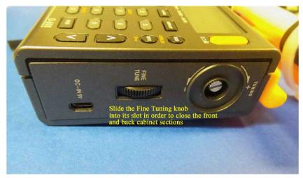
24) Carefully pick up the front and back cabinet sections, and hold the back cabinet section fairly close to the front section (as the radio would normally be oriented, when assembled). Refer to the photo above, and carefully insert the "Fine Tuning" control thumbwheel from the front cabinet section into its slot on the back cabinet section in a sideway movement. This will allow you to fully close the front and back cabinet sections in the next step.
