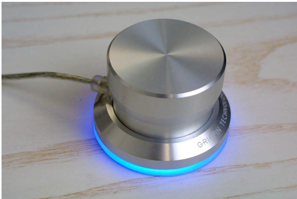
← Fig. 4: The Griffin PowerMate is a stand-alone hardware tuning knob that works with most SDRs
