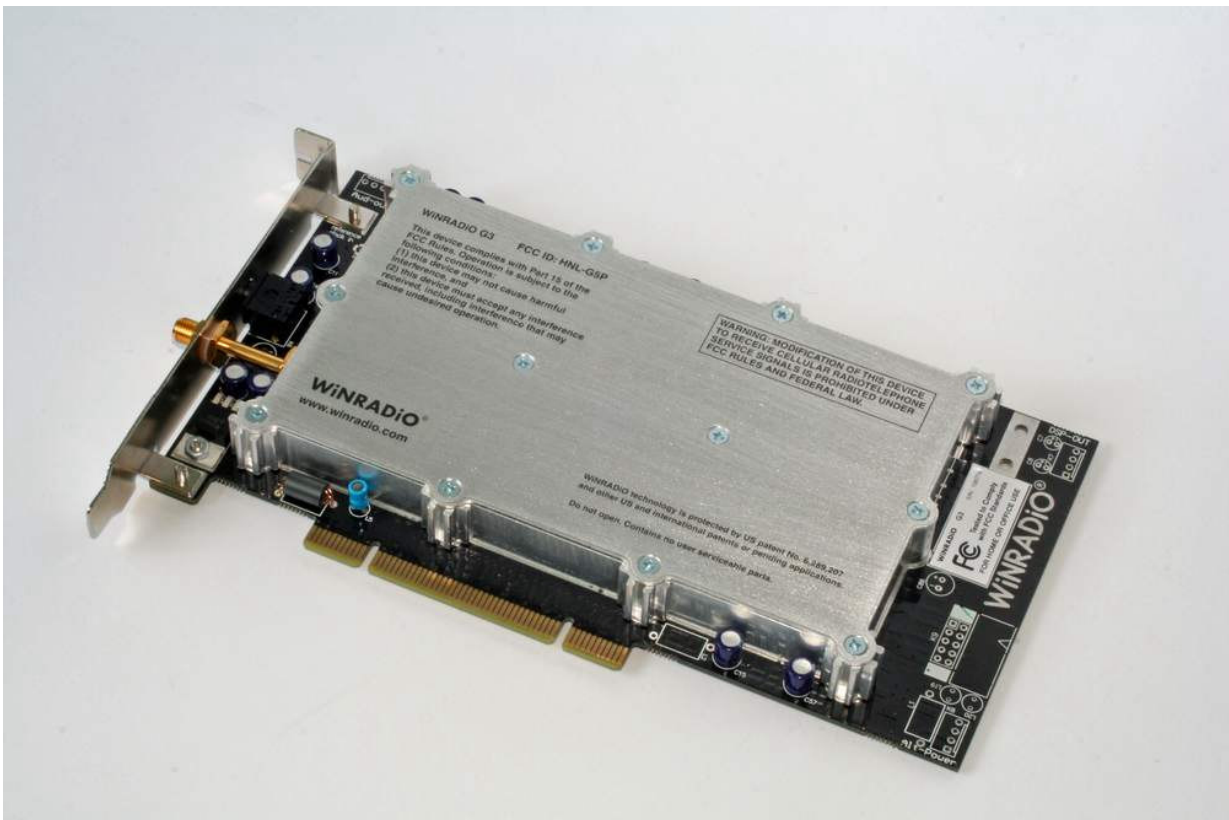
Fig. 2: The G3 series of SDRs from Australian company WinRADIO is available either as external boxes or as PCI cards that plug into one of the expansion slots inside the PC.
