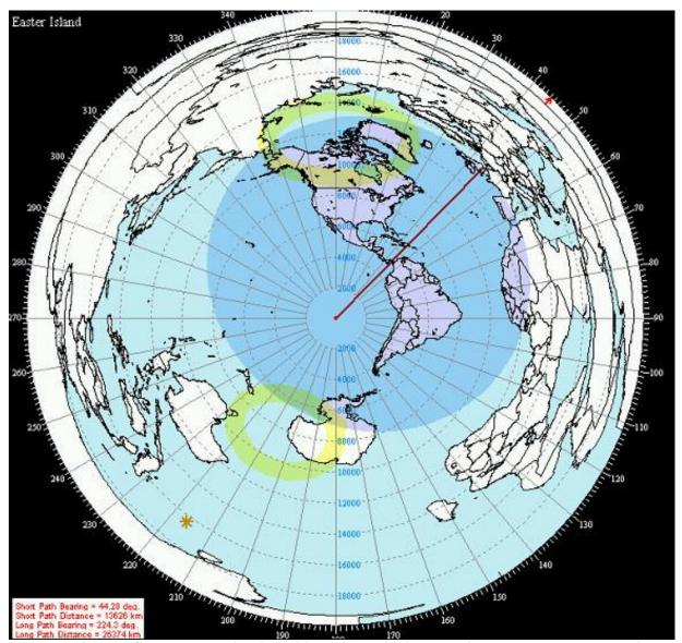
Great Circle map from Easter Island. Red line shows path to London at UK sunrise. Note how Easter Island can "see" most parts of the world without signals needing to pass through polar absorption zones.
