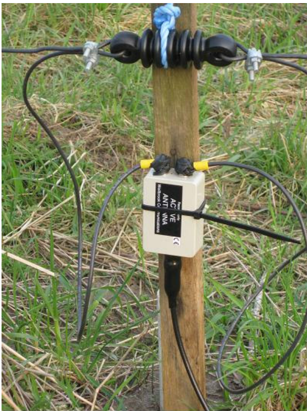
Figure 2: Connections to the Wellbrook ALA 100 head unit
