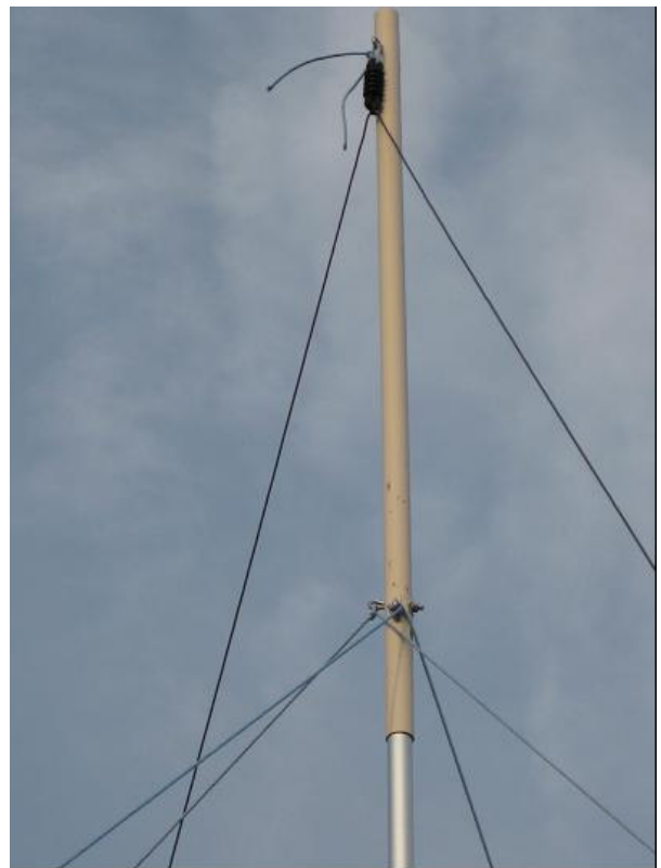
Figure 3 Detail of the plastic piping section at the top of the mast. The wire attached to the upper fixing is the antenna loop
