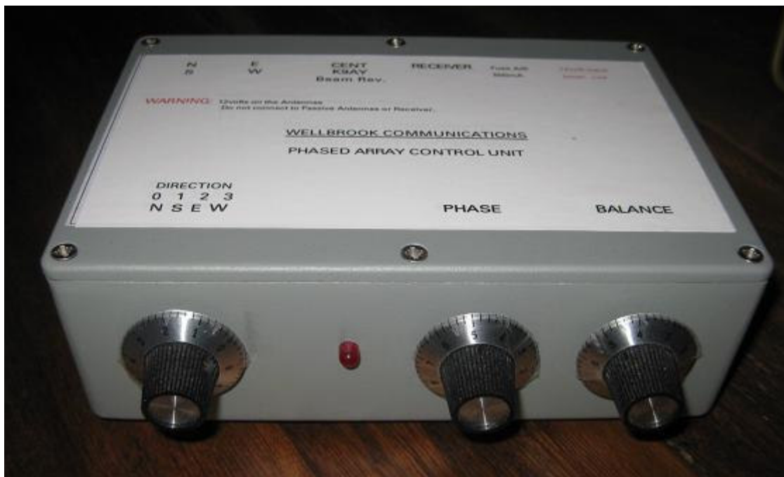
Figure 5; The Phased Array Control Unit.
