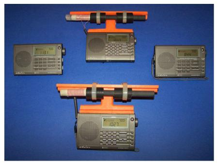
The E100 in stock form is capable of very competitive domestic DX performance, especially on the higher AM frequencies. Its stock IF filter provides it with the best selectivity in the Ultralight radio class, in combination with unsurpassed sensitivity on the X band, and other upper band frequencies. In the recent Summertime Shootout equipment review posted on dxer.ca, it was one of the top two performers, being narrowly edged out by the new
