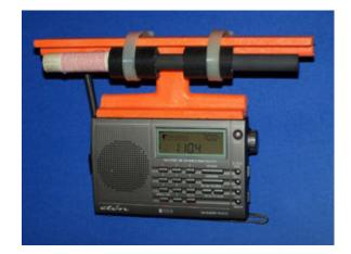
The 7.5" Slider loopstick-equipped E100's have astonishing sensitivity for their size, and have been tested and found fully competitive with RF-2200's, ICF-S5W's and other top AM portables in weak signal capability. Because of the E100's digital tuning convenience and memory capability, however, a Slider-equipped E100 can often exceed these analog portables in overall DXing performance.
