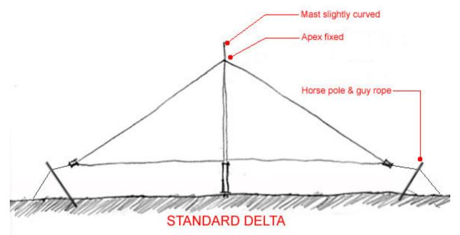
The first antenna drawing is the design that we use for Deltas that are elevated about a meter off the ground: K9AYs, and KAZs, as well as the antenna elements for many of our phased arrays. The top drawing is a typical side elevation of the antenna.
