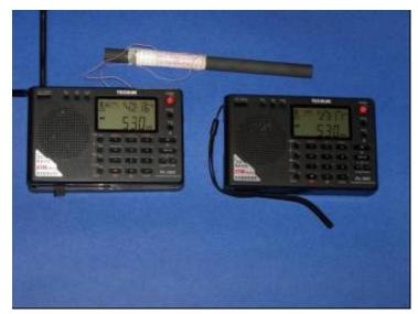
loopstick, but it will also use a 40/44 Litz wire coil found to have the optimal inductance match (with the 4734 DSP chip varactor) for maximum AM sensitivity. In detailed testing with an 81-turn Slider coil and this 7.5" Amidon ferrite bar (shown in the picture to the left), AM signal strength readings were checked on the PL-380's digital display for different coil positions (and different inductances) as the coil was slid across the ferrite bar.
