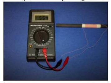
554  $\mu$ h inductance was found to be optimal for a loopstick constructed of a 40/44 Litz wire coil on a 7.5" type 61 ferrite bar in the PL-380 model, recent testing indicates that the changing any of the experimental parameters (ferrite bar size or length, ferrite mix, Litz wire type, coil "Q" or DSP radio model) may result in a different optimal inductance value..
