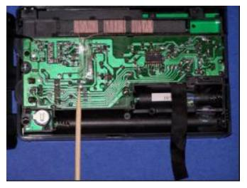
(where the coils meet the plastic slot), it is unlikely to salvage the loopstick intact in one piece, but for purposes of the transplant modification, the empty plastic slot will provide a convenient routing space for the new 40/44 Litz wires, without the stray inductance that would occur if the stock loopstick were left in the cabinet.
