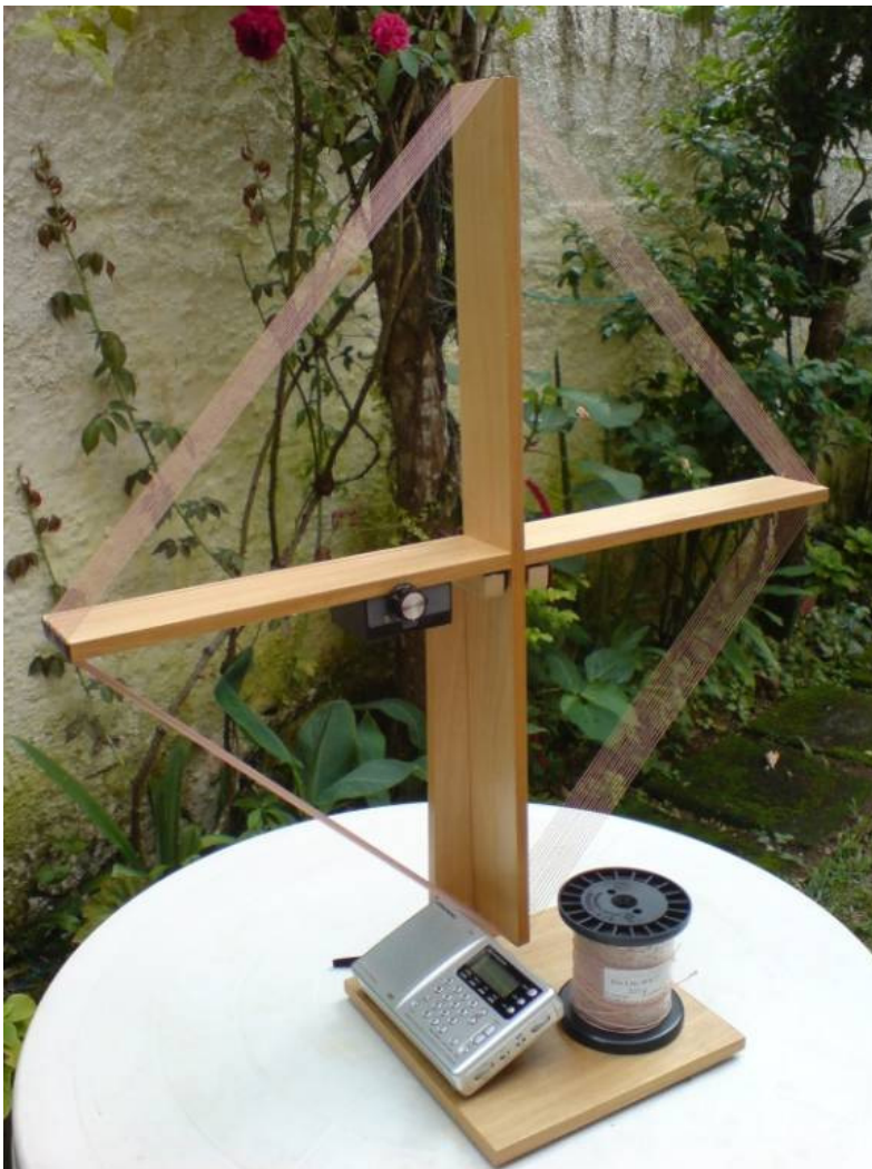
<---Air Core Loop for MW - 100 cm (39 inches) side length of the square with Litz wire coil
