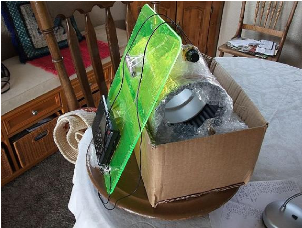
A Ferrite Sleeve antenna in a box coupled to an Ultra-Light Receiver – all easily rotated using a Lazy Susan
