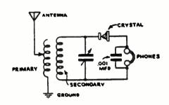
Circuit of a simple crystal receiver
