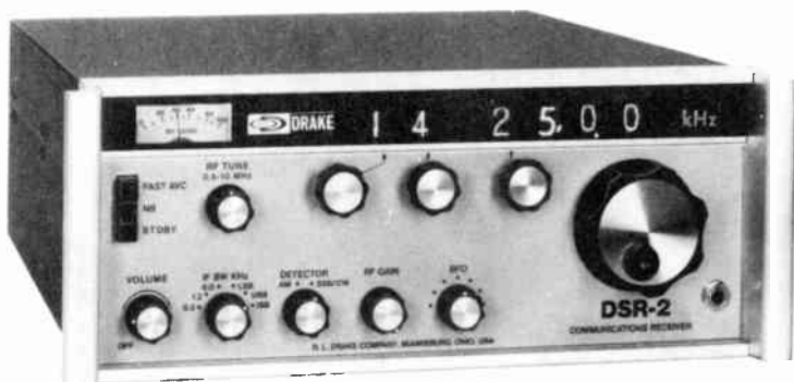
Fig. 4-6 Drake offers this continuous coverage 10kHz to 30MHz digital synthesized solid state DSR-2 as their "top of the line" communications receiver in the $3000 price range.
