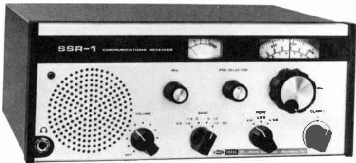
Fig. 4-4 The new Drake SSR-1 is a synthesized, solid-state desk-top 500kHz to 30MHz AM portable. A great new receiver in the $350 class.
