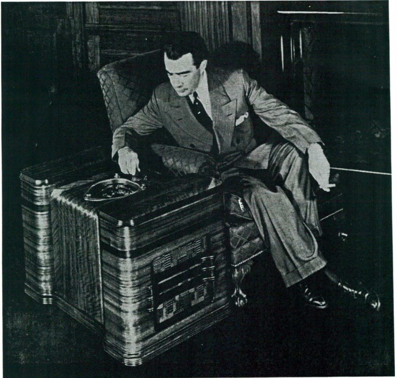
Figure 6. This 1937 photo shows Zenith's founding president, Commander Eugene F. McDonald, Jr. at the controls of the 15 tube "chairside" model 15U246. The chairside was a popular cabinet style derived from the more standard console models of the late 30s. Photo courtesy of Zenith.
