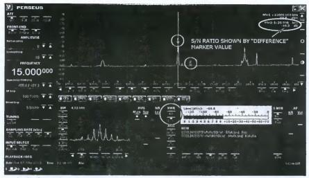
Typical S/N ratio measurement settings for use with the Perseus SDR is shown above. A right-click with the computer's mouse places signal level markers where desired. The "Delta" button under MKR (marker) automatically calculates the real time difference.
