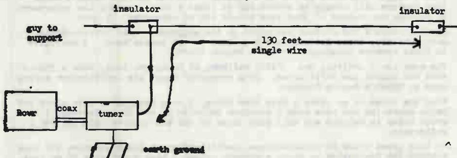
"The secret to this antenna is that you need an antenna tuner and a good ground system. Also the antenna wire should be as high and in the clear as possible. I use an MFJ Versa Tuner which will match just about anything to a 50 ohm receiver input. Many tuners are available from companies like MFJ, and the prices for "bare bones" models are quite reasonable. For a complete catalog from MFJ write: MFJ Enterprises, Inc., Box 494, Mississippi State, MS 39762.
