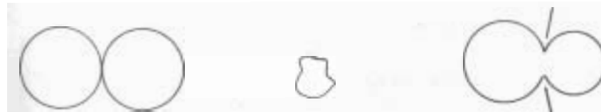
Perfect loop pattern + Electrostatic pickup = Distorted pattern
