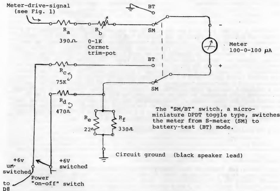
The trim-pot is used to adjust for a full-scale-left deflection on the meter with zero-signal received. Tuning the receiver above 1600 kHz. will provide a nearly-zero signal level under most conditions.
