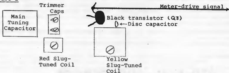
The meter-drive-signal measures approximately  $+0.5$  volts for zero-signal and about  $+0.2$  volts for full-scale signal (a strong local).
