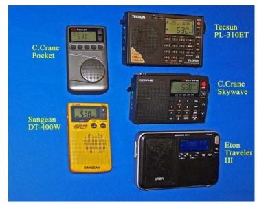
innovative Si4734 DSP chips were introduced by the Kchibo and Tecsun companies in 2009 the AM band selectivity of pocket radios was dramatically increased, although such models came with congenital quirks such as internally-generated heterodynes. For about four years DXers wondered when a manufacturer would solve this problem, and introduce a pocket radio with both excellent DSP selectivity and freedom from bogus heterodynes. That wait is now over – such a radio is now an exciting reality.
