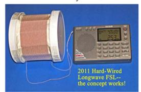
validity of the hard-wired FSL concept was proven to my satisfaction (see photo at left). The challenge has always been to create a hard-wired FSL that would offer both high MW sensitivity and lightweight portability – a value tradeoff that made this project especially intriguing.
