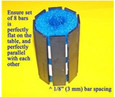
mm) spacing between the bars. Continue to place the other 6 bars on the inner foam core in exactly the same way, ensuring that all 8 bars are flat against the table and parallel with each other, having 1/8" (3 mm) spacing between them. If necessary (after placing all 8 bars on the tape), even out the spacing by moving certain bars slightly so that the gaps between them are all equal. The set of 8 bars will be compressed in the next step to form an octagonal pattern.
