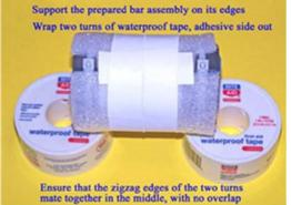
11. Refer to the photo at left. Support the edges of the prepared bar assembly so that it will be raised off of the table. Wrap two turns of the 1" waterproof tape tightly around the center of the prepared bar assembly, adhesive side out (as shown). When wrapping the second turn, ensure that the inner zigzag edge of the waterproof tape mates evenly with the inner zigzag edge of the first turn of tape, with no overlap or gap.
