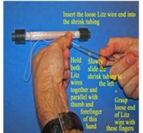
end of the Litz wires through the shrink tubing until about 3 inches of wire extend from the tubing. Carefully insert the other end of the Litz wire through the shrink tubing, and use the procedure (and photo) in Step 30 of the Loopstick Transplant article to run the second Litz wire through the shrink tubing, as shown. The related photo for that procedure is included at left.
